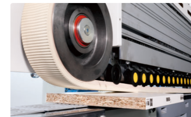
履带压料 Top presser by v-belt
