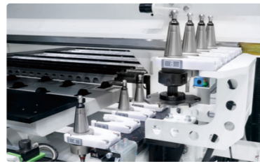
八刀位自动换刀刀库 ATC 8 by servo
