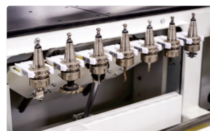
七刀位自动换刀刀库 ATC 7 by servo
