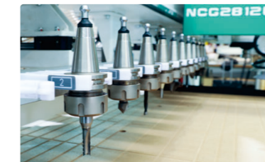
12刀位自动换刀刀库 12-slot line tool changer
