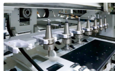
ND712DTL配置2组8刀位自动换刀刀库 2 sets 8-slot tool magazine of NCB612DPTL
