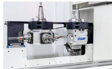
双刀位自动换刀刀库 ATC 2 by servo
