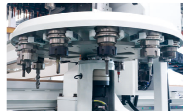
12刀位伺服换刀刀库 ATC 12 by servo
