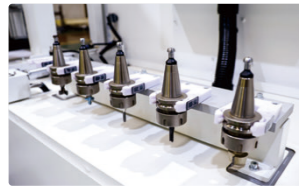
六刀位自动换刀刀库 ATC 6 by servo
