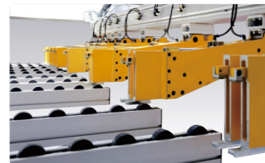
配置10个工夹 Configured with 10 sets of grippers
