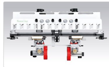
伺服水平齐头 Servo controlled flat end cutting
